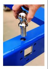
B) Fasten the tow ball to the HOOK-BASE: first apply a lock washer to each bolt; then apply a hex nut. Fully tighten the nuts to secure the connections.
