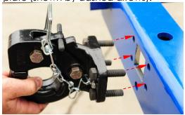
B) Fasten the pintle hook to the HOOK-BASE: first apply a lock washer to each bolt; then apply a hex nut. Fully tighten the nuts to secure the connections.
